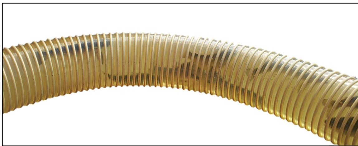
Figure 1.2-3. The behaviour of smolts during pumping can be monitored through a transparent hose. Photo: Å. M. Espmark
