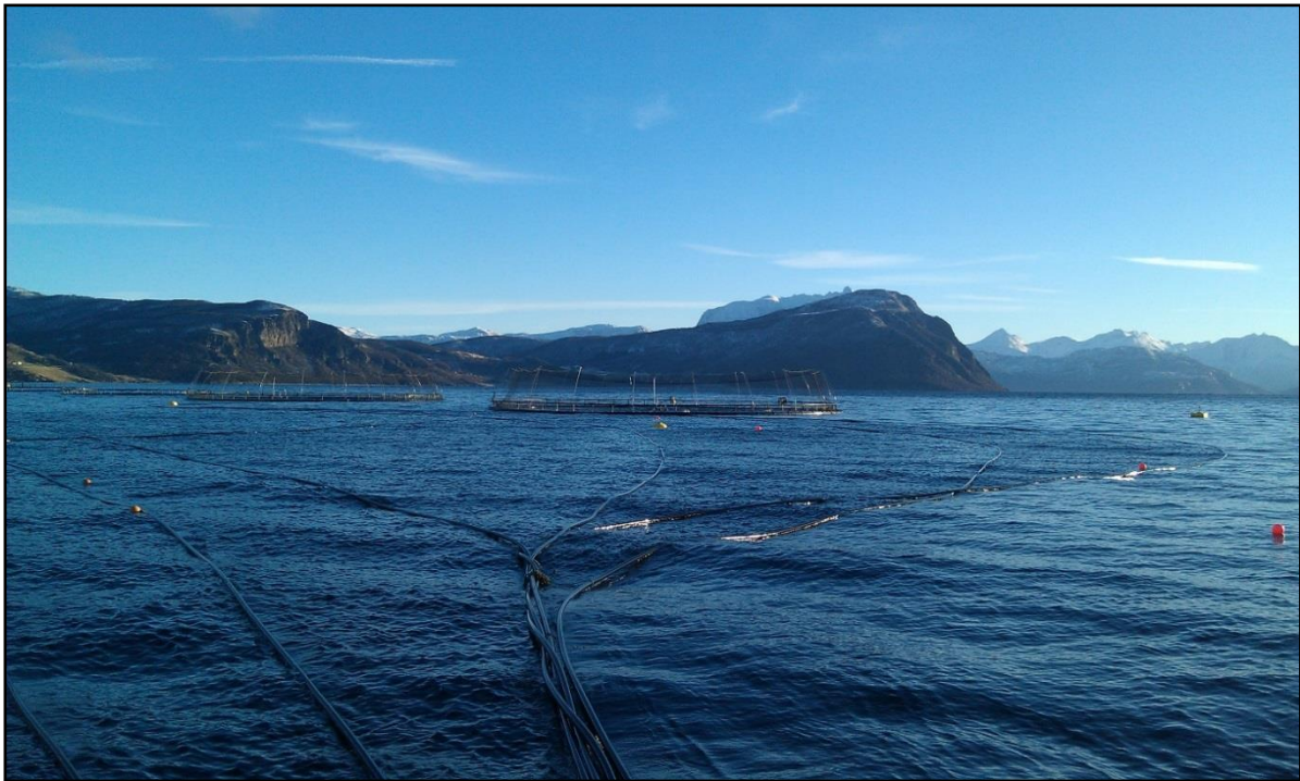
Figure 1.9-1. Feed delivery pipes going from the central feed barge to commercial rearing cages. Photo: C. Noble
