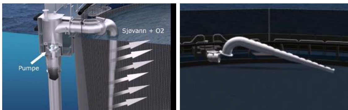
Figure 3-7. The articulating inlet on the Ecomerden CCS
