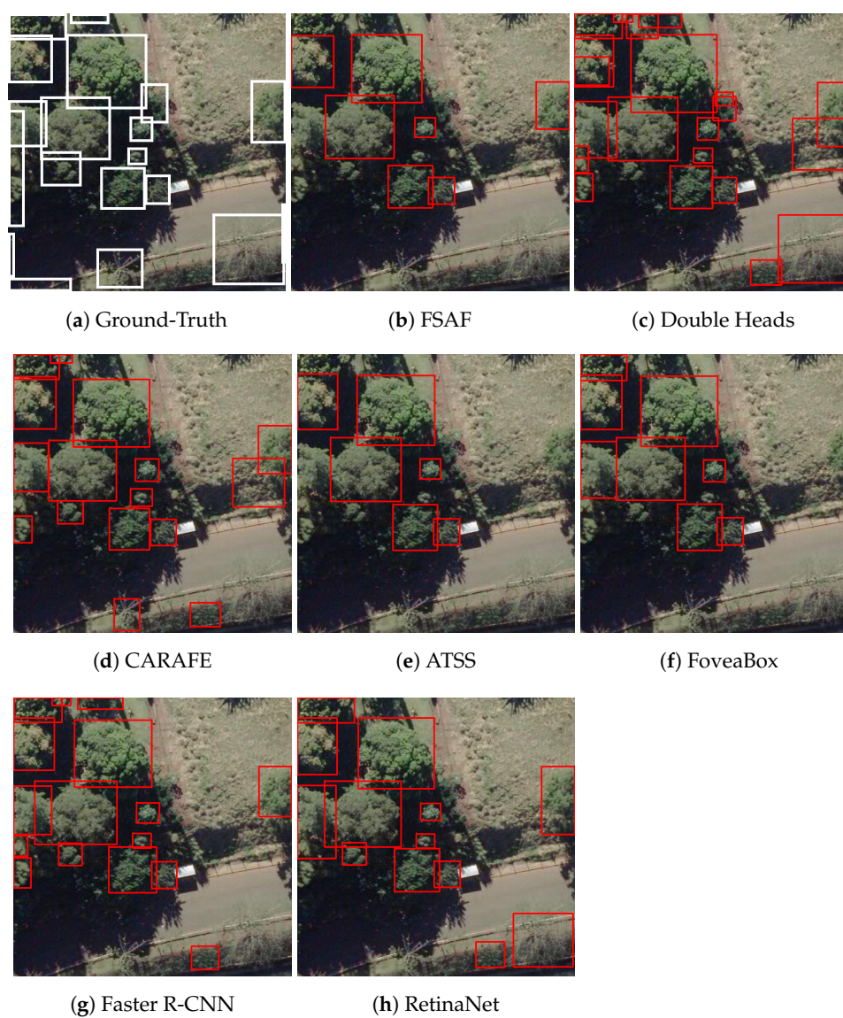
Figure 15. Tree detection with the top five methods, RetinaNet, and Faster R-CNN: performance in a challenging illumination scenario with shadows.
