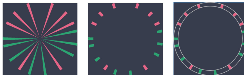
Fig. 7 Wedge pattern (left), bar pattern with the segments arranged orthogonally to the imaginary circular path (centre), and ring-bar pattern (right) stimuli. Bar patterns can be created either from wedge patterns by removing figurality (global orientation information consistent with a figure/shape) through removal of the inner section of the circle (i.e., shortening the segments) or by symmetrically segmenting radial-frequency patterns such as those used by Wilson and Wilkinson (2002). Ring-bar
