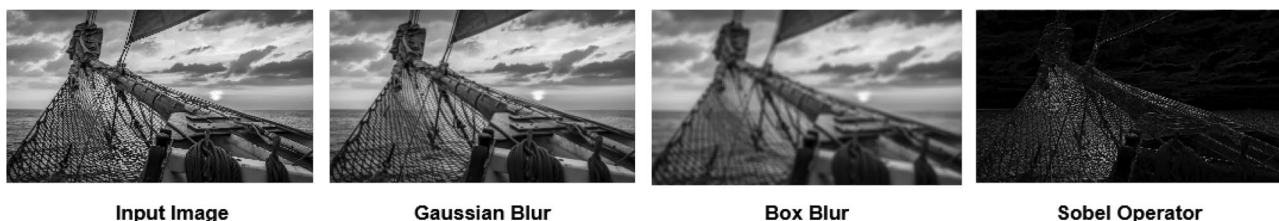
Figure 6 Filter Algorithms Applied onto Input Image.
