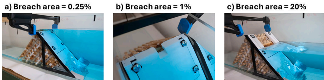
Fig. 6. Photos of the Gapflow Dam models. Water flows from right to left.
