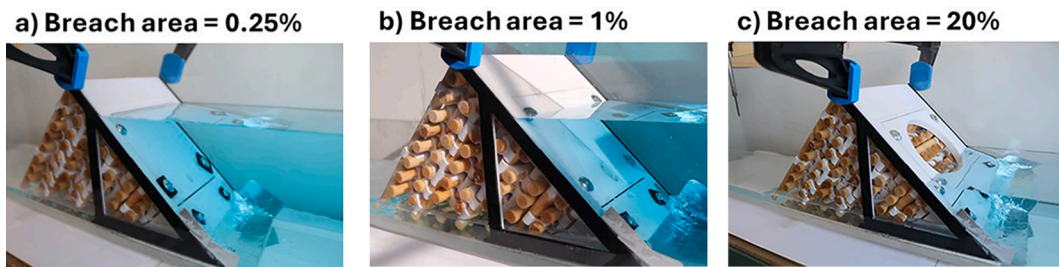
Fig. 8. Photos of the Underflow Dam models. Water flows from right to left.
