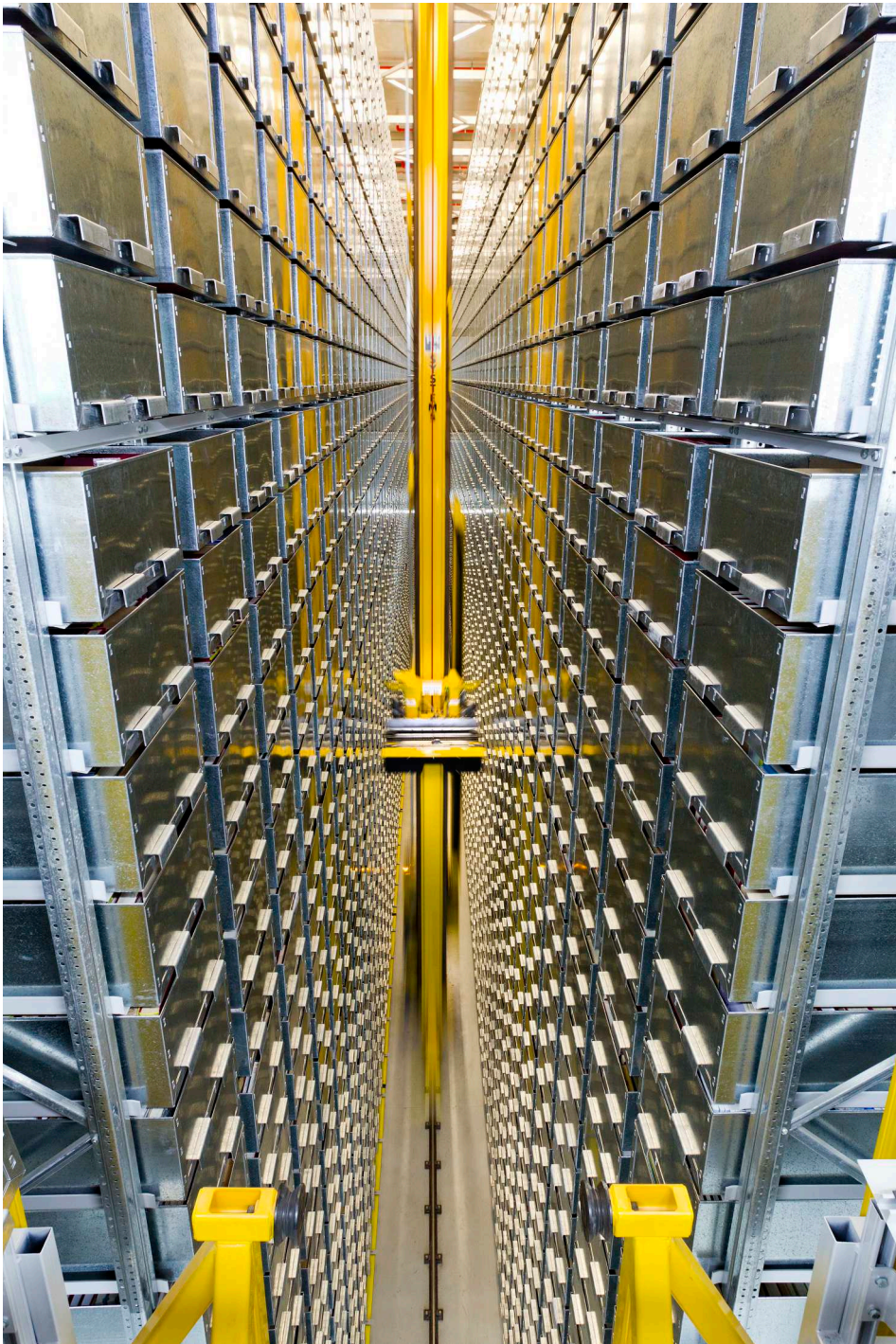
Figure 2. Waranara Library's automated retrieval system. Photo by Paul Wright, used with permission.
