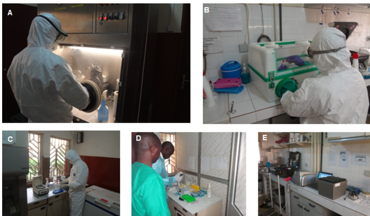
Figure 1. Laboratory set up. (A-B) room for sample inactivation, glovebox in B used in case of power failure and in field deployment, (C) room for RNA extraction, (D) Room for master mix preparation (E) room to add sample RNA to the master mix and to run the real time PCR.
