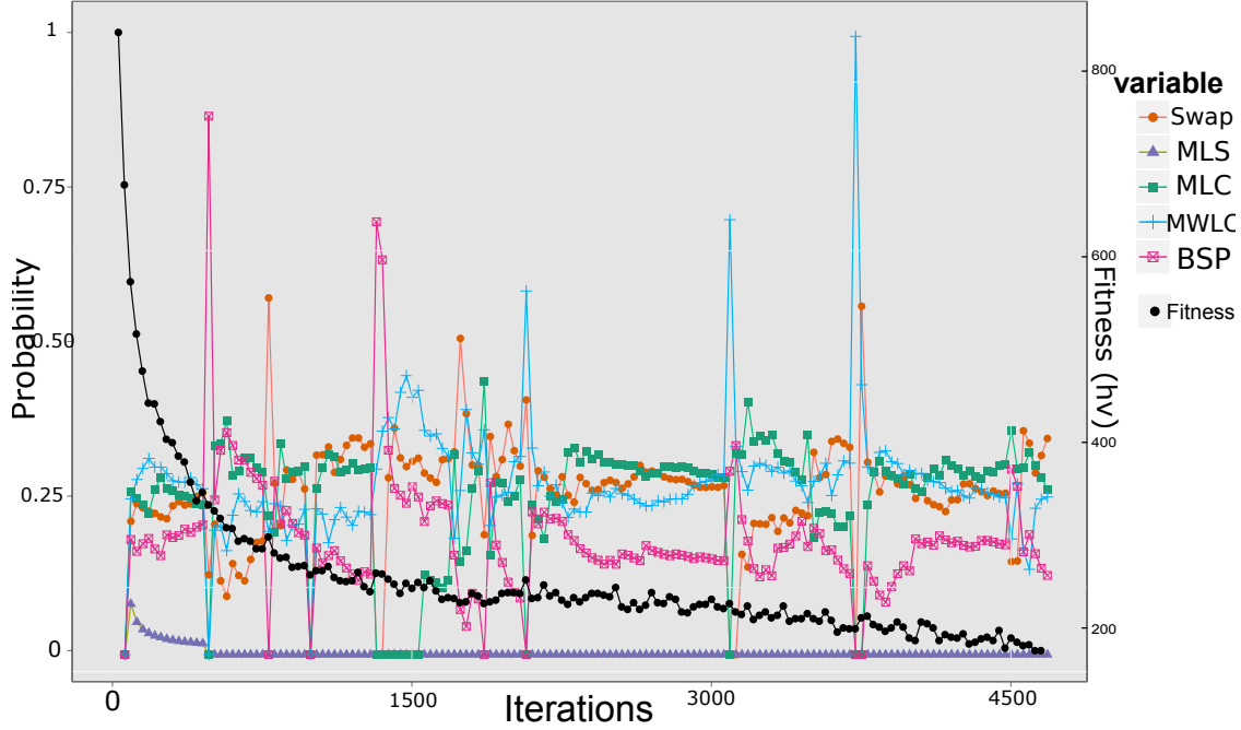
Figure 3: Course timetabling, ITC-2007 instance 1: Operator selection dynamic with the selected sub-set of 5 heuristics. Curves show probabilities over time. The fitness over time is also displayed (black line)
