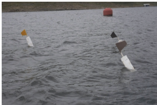
Figure 12: Drogues deployed in Lake Volta
