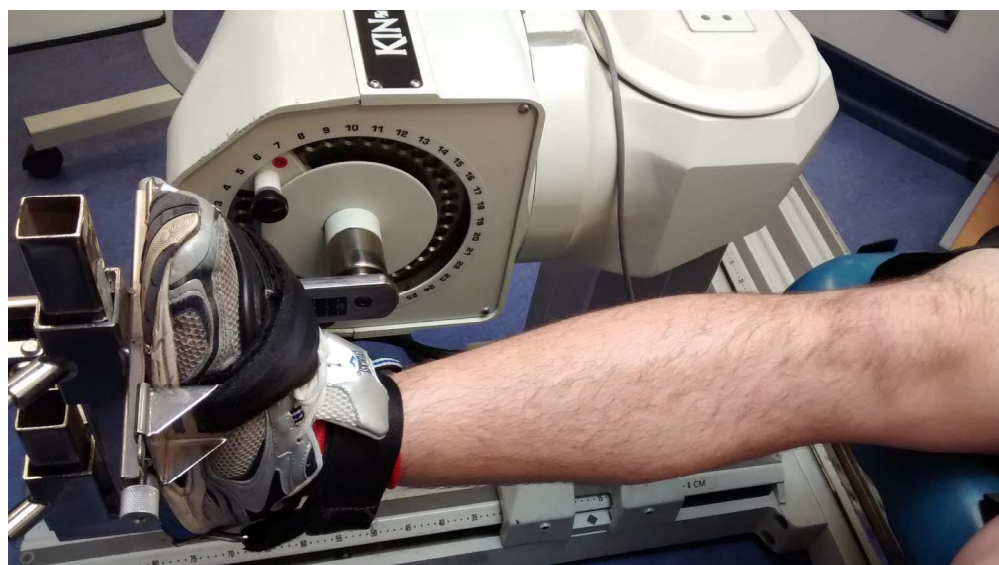
Figure 3. Isokinetic dynamometer setup for PMT and MVC assessment. Ankle flexed at 90° relative to the tibia. 342x192mm (300 x 300 DPI)
