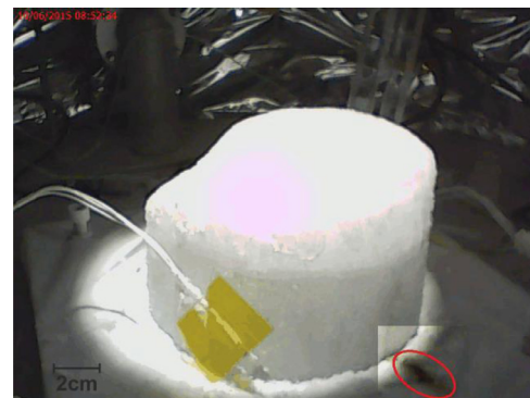
Fig. 5. Dust deposit obtained from dust seepage. The deposit, visible at the lower right of the ice block, was approximately 2 cm long and about 0.7 cm at its broadest extent, so much smaller than the fan-shaped deposits seen for the other experiments. The picture was taken at the end of the first irradiation phase.
