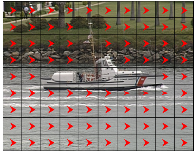
Fig. 3 Motion block estimation.
